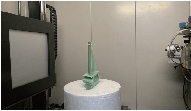
图2 某燃气轮机空心透平叶片蜡模工业 CT 检测原理图 Fig.2 Schematic of industrial CT detection of hollow gas turbine blade wax mold
